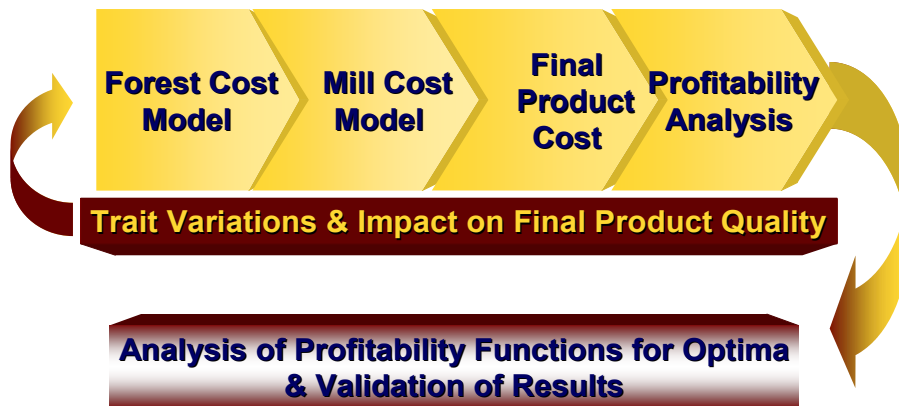
Figure 2: Approach to model wood and fiber properties on the cost of slush pulp, linerboard and mill profitability (15).
